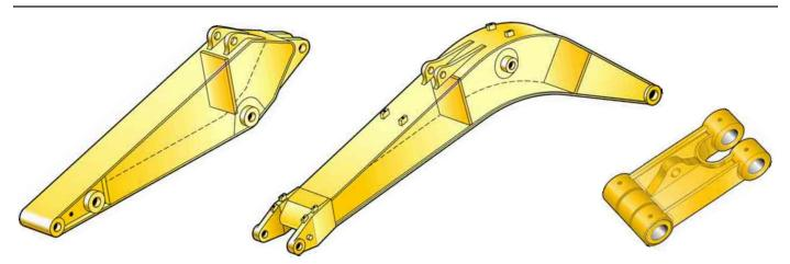
Front Linkage Attachments. Select the right combination of front linkage with your Cat dealer to ensure high productivity from the very start of your job. Three types of booms and four sticks are available, offering a range of configurations suitable for a wide variety of applications and offer a large combination of reach and digging forces for optimum versatility. All booms and sticks undergo a stress relieving process for greater durability.
